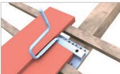
Position of the bracket with beavertail tiling
